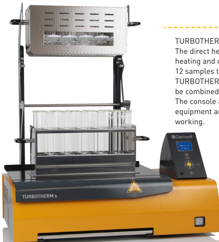
TURBOTHERM is a digestion unit based on infrared technology. The direct heat input by infrared radiation provides short heating and cooling times: Only 10 minutes are needed to bring 12 samples to boil.
