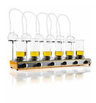
Combined apparatus for classic, manual acid hydrolysis.
